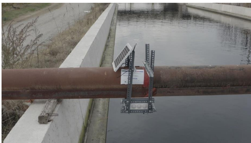
Figure 18: RiverMon low cost IoT water level sensor.
